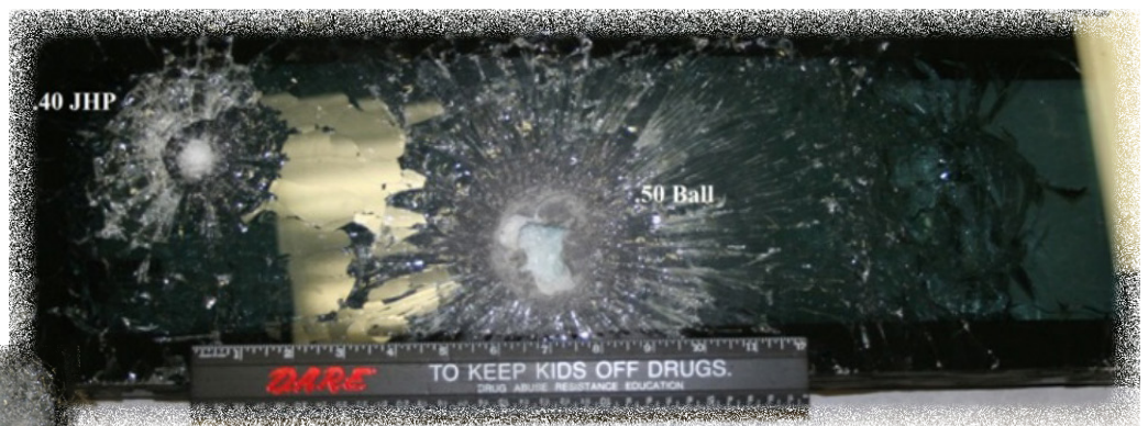
The firearms examiners evaluated the performance of ballistic glass from a BearCat armored vehicle. These photos show both sides after impact.
