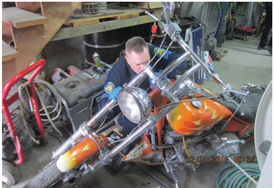
Cpl. Nate Bradley, Troop A, performs an acid restoration on an altered motorcycle frame.
