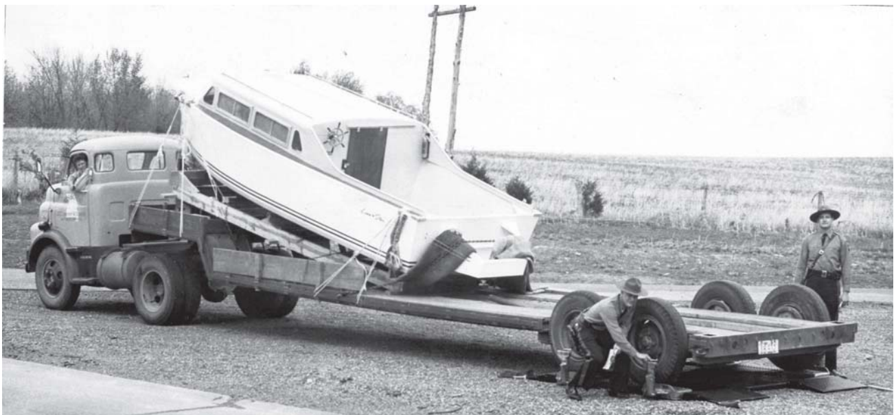
Portable scales are used to check the weight of this tractor-trailer. P.V. Volkmer is on the right.
