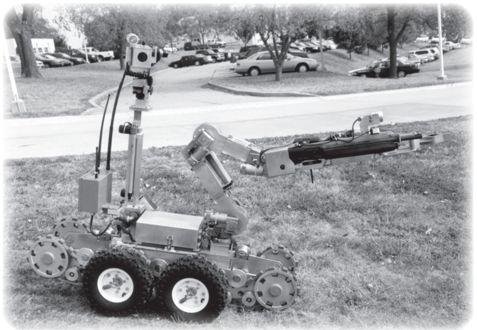
This Remotec F6A robot allows technicians to render bombs safe from a distance.
